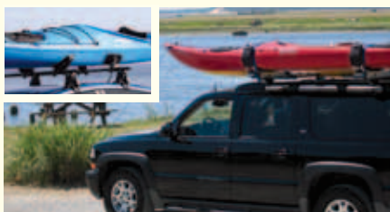
Right-side up using a Hullavator, inset using saddles
