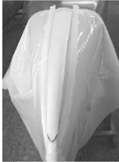
Skid plate ready for resin application
